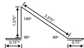
The schematic drawing below illustrates the dimensions to fabricate the rail from the same material as the roof.
