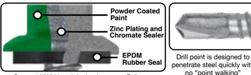
Cupped HWH head design improves Pull over strength versus standard HWH & Bonded Washer. ST Fastening Systems sockets are designed to allow for the added thickness of the powder coat.
