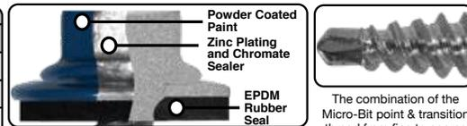
Hex Washer Head with EPDM rubber washer provides a watertight seal on roof applications. ST Fastening Systems sockets are designed to allow for the added thickness of the powder coat.
